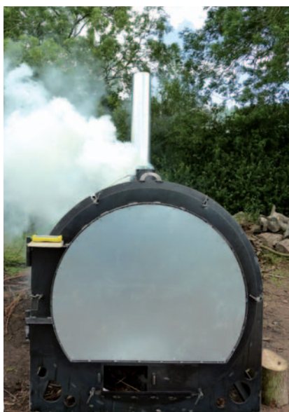
The Exeter Retort filled with lengths of small diameter branchwood (right) ready to be lit. Initially steam is produced by the heat (above), but as the temperature rises so volatile gases are emitted and are burnt off inside the fire chamber. The retort takes material it would be difficult to manage (top) in metal ring kilns
