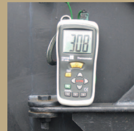
Once the temperature in the kilns reaches 300° the gases begin to escape through pipes underneath the kiln. By capping these pipes volatile gases are redirected into the fire chamber to raise the heat to 600°
