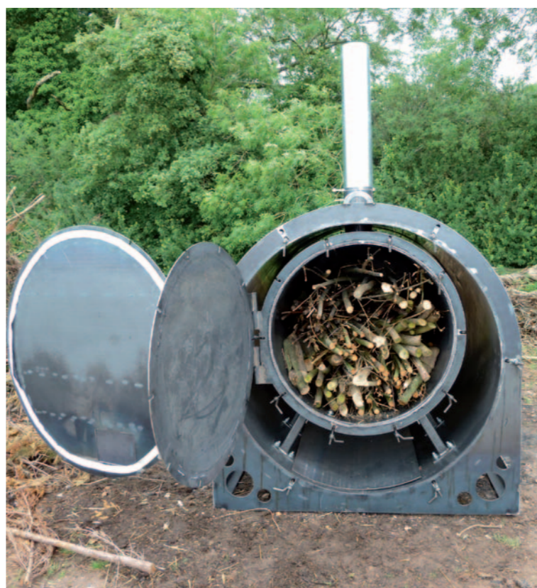
The Exeter Retort filled with lengths of small diameter branchwood (right) ready to be lit. Initially steam is produced by the heat (above), but as the temperature rises so volatile gases are emitted and are burnt off inside the fire chamber. The retort takes material it would be difficult to manage (top) in metal ring kilns
