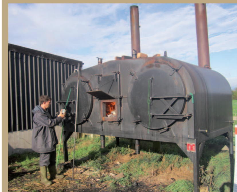
Tim Smith checking the temperature in one of the Pressvess kilns. Notice the lack of smoke coming out of the chimneys. Retorts produce much less pollution
