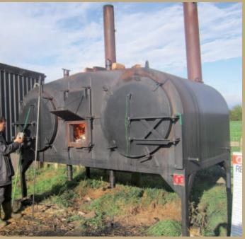
im Smith checking the temperature in one of the Pressvess kilns. Notice the lack of moke coming out of the chimneys. Retorts produce much less pollution
